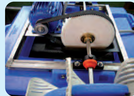
detail: motor with belt drive
